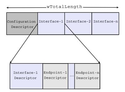
Figure 9.1: Configuration descriptor with interface and endpoint descriptors
