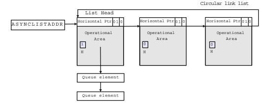
Figure 5.3: Asynchronous queue in host controller
