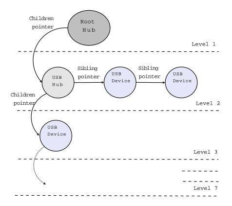
Figure 9.2: USB tree topology as maintained by USB manager
