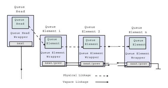
Figure 8.1: HCD asynchronous queue management overview
