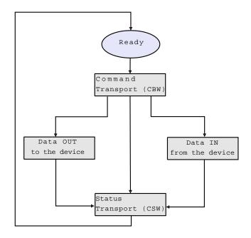
Figure 10.1: Command/Data/Status Flow
