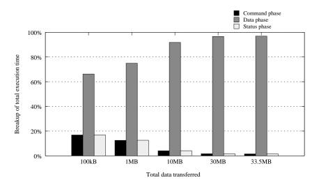
Figure 11.5: Break up of time spent in read command request stages The Linux reports 13 MBps bandwidth with dd command utility on the
