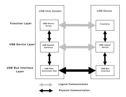
Figure 4.2: Communication flow in a USB system
