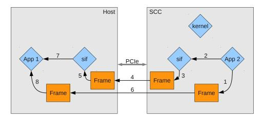
Figure 4.2: Sending of a message from SCC to host
