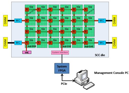
Figure 2.1: SCC Top-Level Architecture
