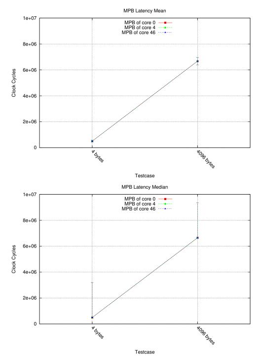
Figure 2.3: SCC MPB memory read times
