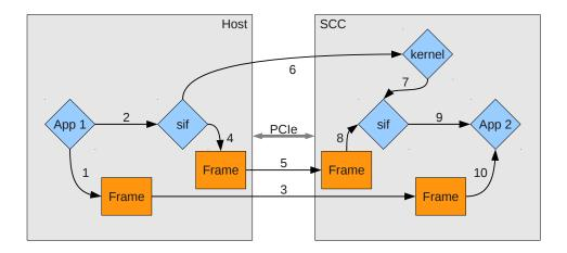
Figure 4.1: Sending of a message from host to SCC
